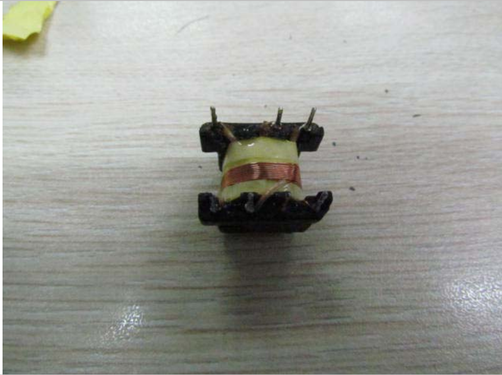
Transformer view of mains power board
