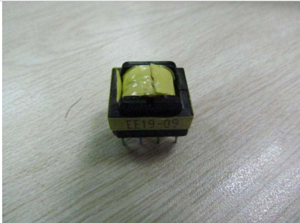
Transformer view of mains power board
