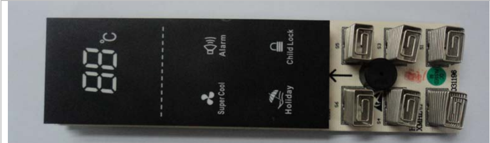
PCB view of control panel
